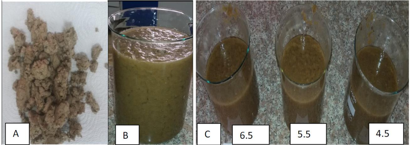
**Fig. 3 :** cellulosic garbage A-Grinding B- garbage with dilute acid after boiling C- PH value
