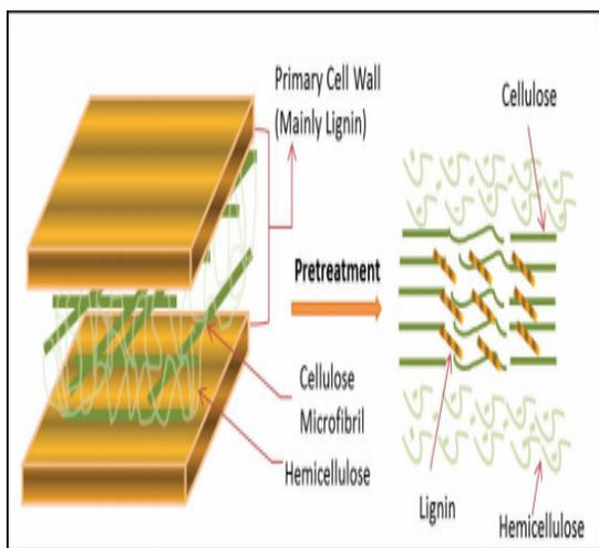
**Fig. 2:** lignocellulose is mainly made up of lignin, hemicellulose, and cellulose fibers
